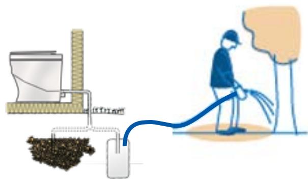
Infiltration    Tank/bucket or Ejektortank
